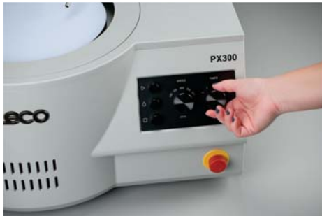
Control panel for controlling wheel speed, water spigot, and timer.
