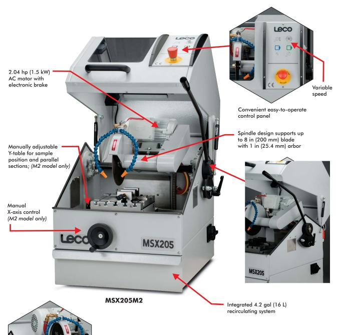
8.26 in (210 mm) x 8.26 in (210 mm) T-slotted table for flexible sample fixturing; table vise included
