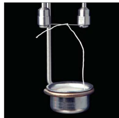
Optional string-ignition combustion vessel provides a seamless analysis without fuse wire connections.
